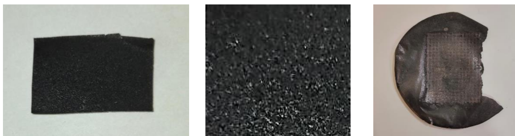
Figure: (a) fabricated adsorbent pad, (b) magnified area on the pad indicating porosity, (c) high brittleness of one of the membrane design
